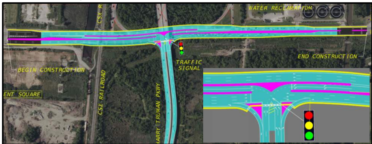
Figure 22: Alternative 2 – Elevated Green-T Intersection
